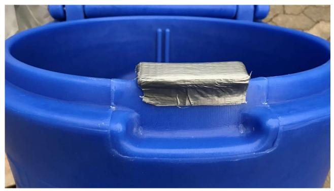
Alternatively, to screw extra material onto the counter rail, for example a small piece of plastic, or just some screws (the photo shows some small plastic that are placed there after pre-drilling holes for them):
